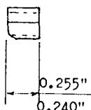
X.36. Outer Pawl for Sliding Carrier of X & FX.
