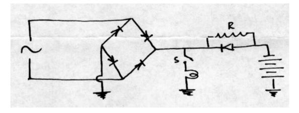
When closing switch S with the cycle stationary, the battery pack (3 x R20) supplied the filament lamps. As the cyclist increased speed, the dynamo would generate, sharing the load until at 9mph the dynamo took over. Reducing speed the opposite occurred. There was always a light.
